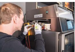
The Convotherm mini's service-friendly design, encountered at every turn, features four service ports and makes servicing and repair easier, faster and more cost effective.
